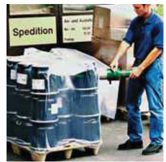
Flameless shrink-wrapping of pallets and bulky goods with the FORTE S3. This allows work to be carried out in closed spaces.
