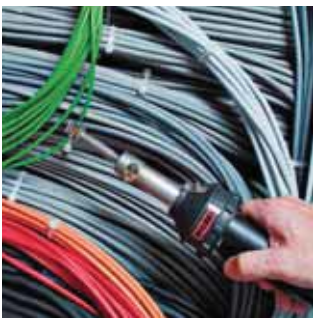
Fitting a solder shrink connection with the HOT JET S and a push-fit sieve reflector.
