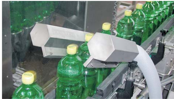
The combination of blow-off nozzles and blowers allows fast and efficient drying of beverage bottles.
