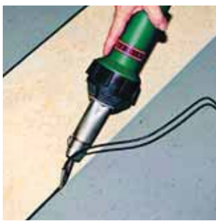
The TRIAC S hand tool, used for welding linoleum, equipped with a speed weld nozzle.
