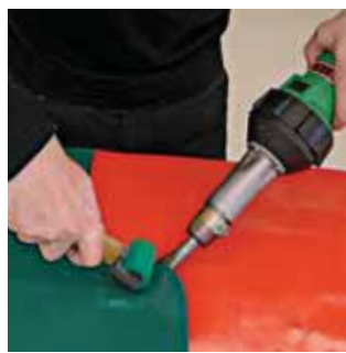
TRIAC PID: monitoring of welding temperature for top quality.
