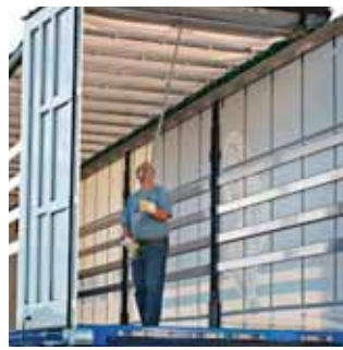
Tarpaulin bows for fixed and sliding rooftops of lorries (Picture: Krone).
