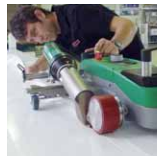
Very easy hem and piping welds with the hem/pipe welding kit.
