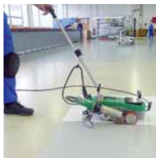
Constant, wrinkle-free overlap welds.
