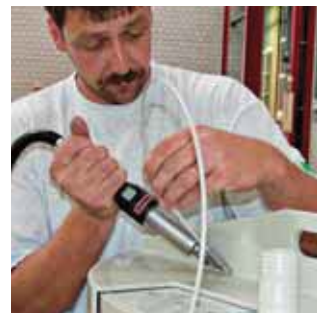
Wire welding using the compact and light WELDING PEN R.
