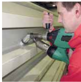
The 45° angled adapter for the WELDPLAST S2 facilitates welding in difficult positions. (accessory)
