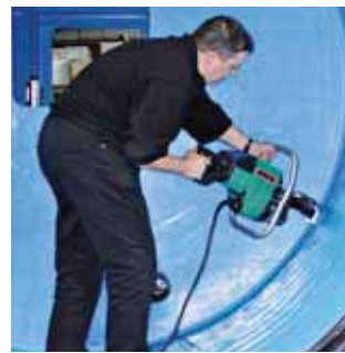
The WELDPLAST S6 is guided easily with the practical control wheel grip.
