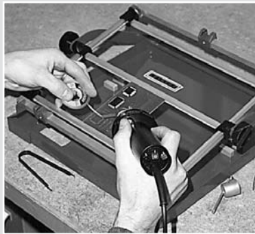
Removing excess solder with hot air and de-solder braid.
