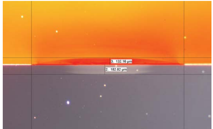
Section through a laser welding seam of 3 mm width.
