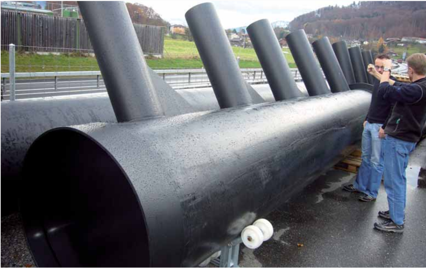
▲ Pipe constructions made of PE for thermal energy systems, Switzerland.
