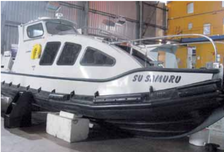
Ship constructed completely of HD-PE, Turkey
