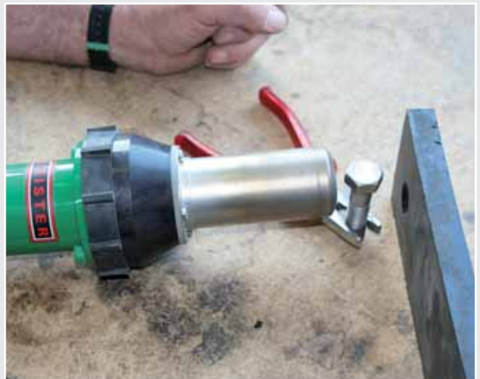
Heating a hex bolt before plunging.
