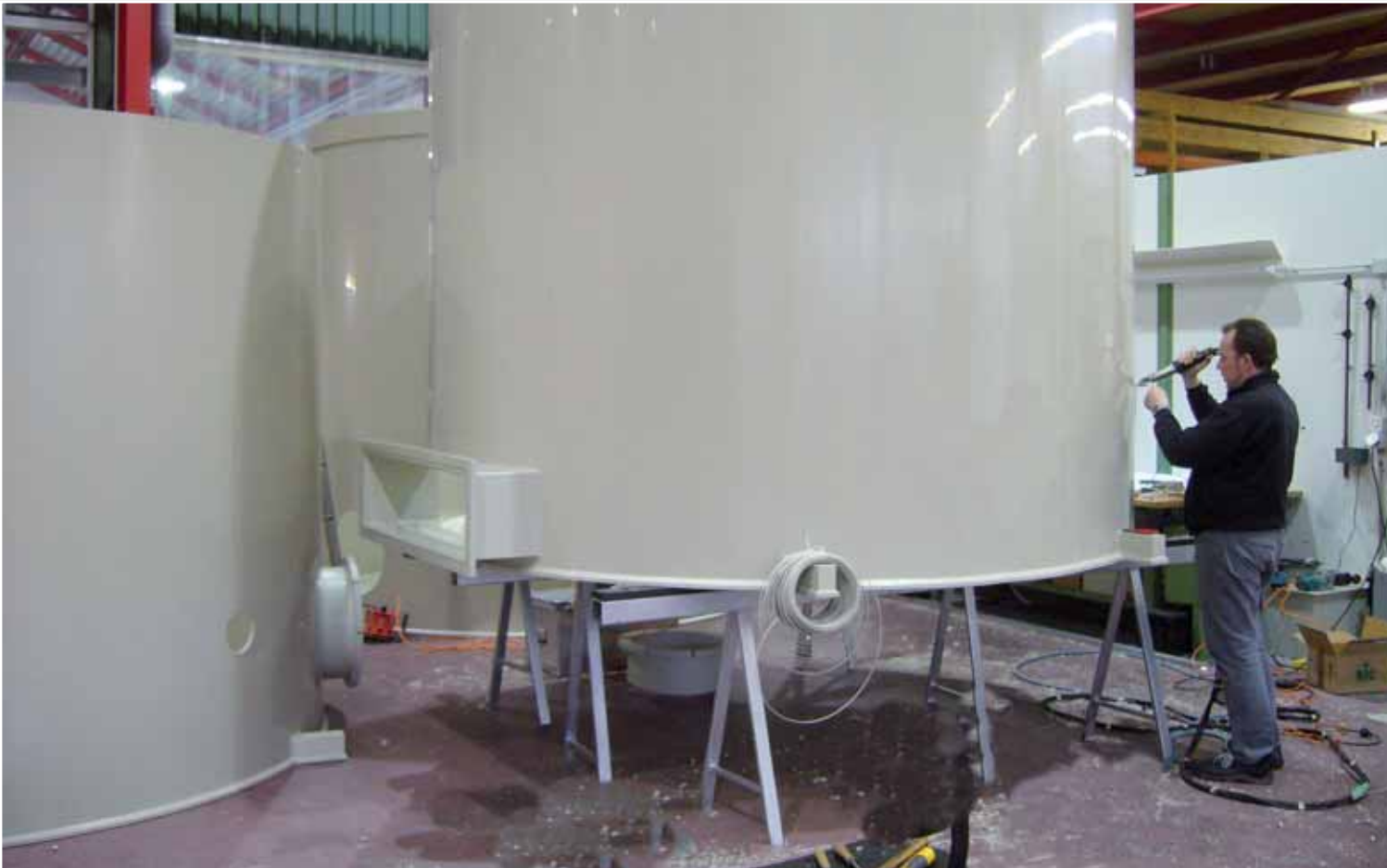
▲ Pipe constructions made of PE for thermal energy systems, Switzerland.
