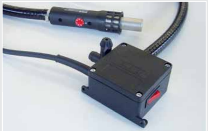
Connection to air supply with the connection box.
