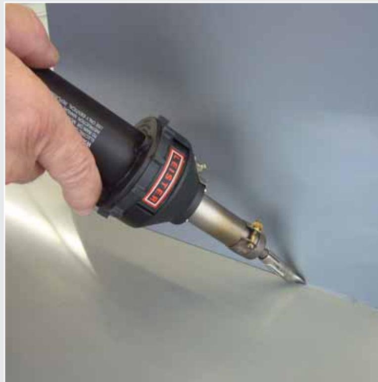
HOT JET S in use for stitch welding.
