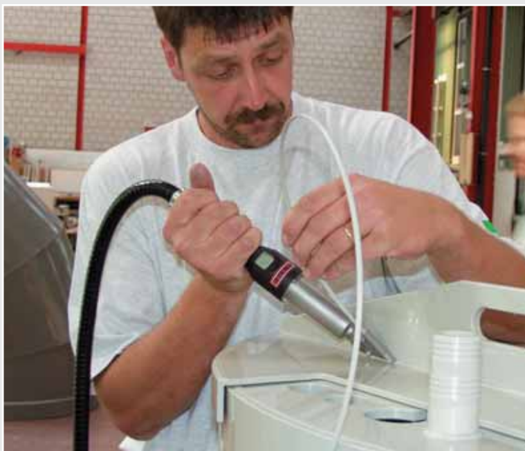
Rod welding using the compact, powerful WELDING PEN R.
