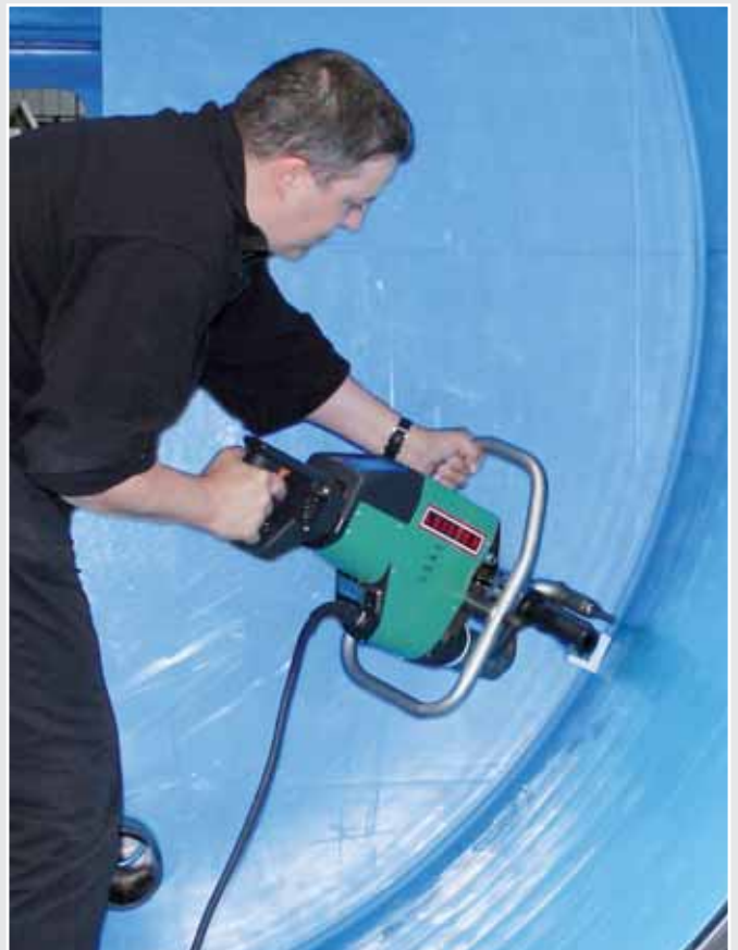
The WELDPLAST S6 is guided easily with the practical control wheel grip.
