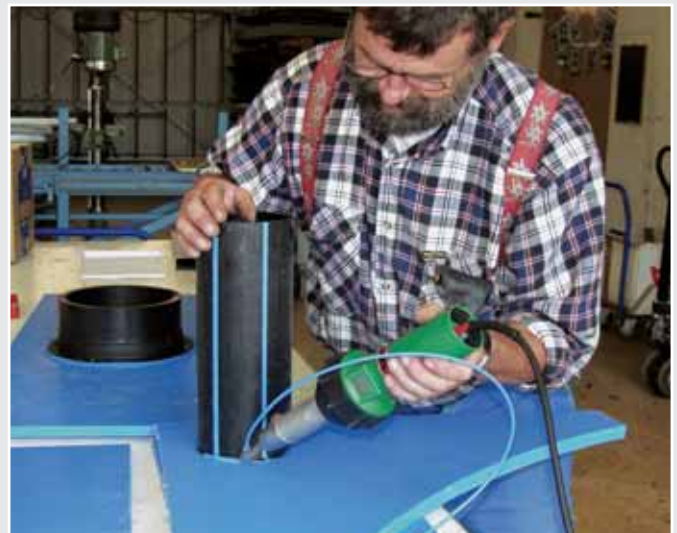
TRIAAC PID: Controlled welding temperature for a perfect quality.
