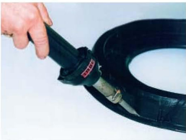
HOT-JET S being used for PE-HD tacking.
