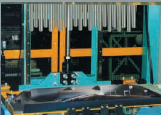
LEISTER heater Mini used in an installation for riveting door side claddings.
