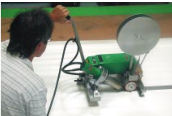
Welding of a 50 mm webbing onto a truck cover. The UNIMAT guarantees a high welding speed.
