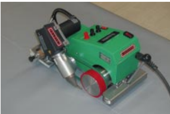
UNIPLAN used for overlap welding of a truck cover. Welding speed about 7 m/min. (23 ft/min).
