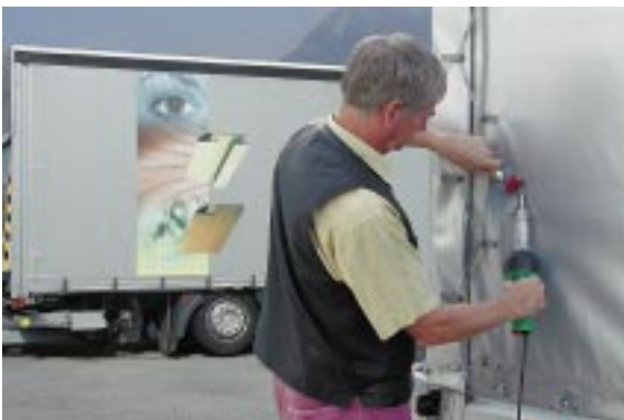
TRIAC PID with 20 mm wide slot nozzle and pressure roller being used for repair welding on a tarpaulin.
