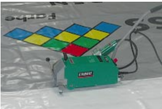
20 mm overlap welding of a truck cover using the UNIMAT. Welding speed up to 12 m/min. (40 ft/min).
