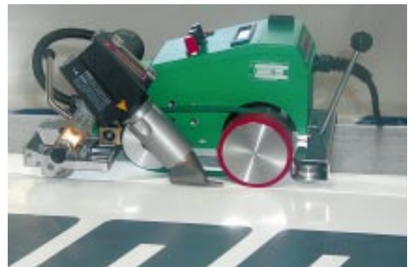
Problem free flat hem weld using the UNIPLAN
