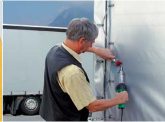
Repair welding of a truck tarpaulin using TRIAC PID with wide slot nozzle and pressure roller.
