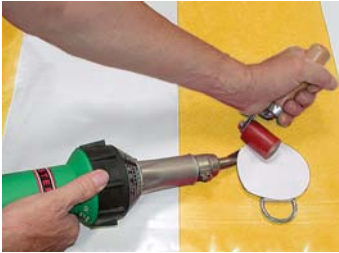
Welding tie downs with TRIAC S.
