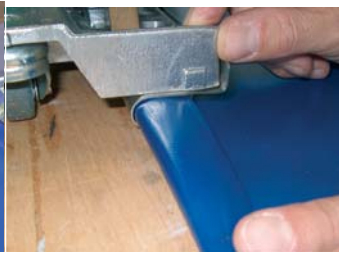
Hem welding with the UNIPLAN E.
