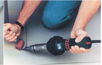
TRIAC PID with a 20 mm wide slot nozzle and pressure roller used to weld plastic roofing membranes.
