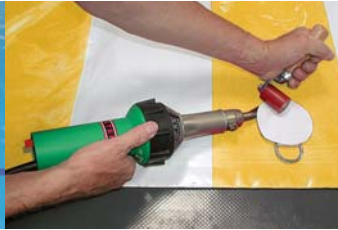
Welding tie downs with TRIAC S.
