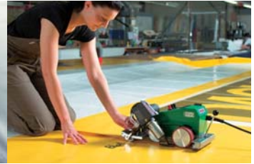
Overlap welding of a billboard with UNIPLAN E.
