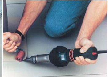
TRIAC PID with a 20 mm wide slot nozzle and pressure roller used to weld plastic roofing membranes.
