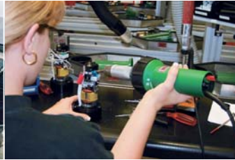
Shrinking a solder sleeve with TRIAC PID.
