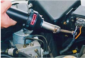
HOT JET S with spoon sieve reflector for solder shrinking.
